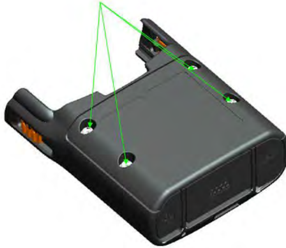
Figure 12-15 Tightening Back Housing
