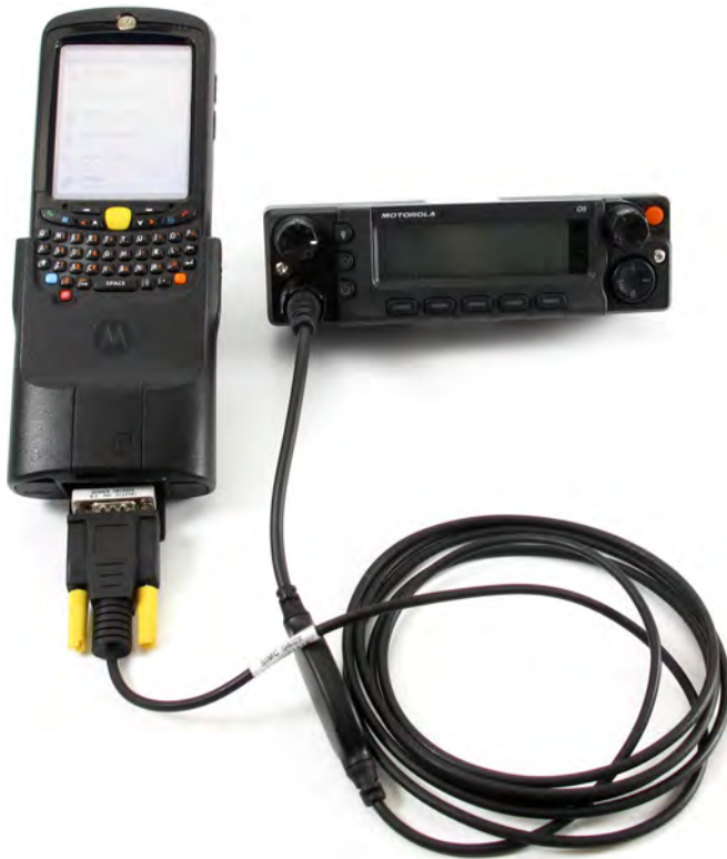
Figure 8-1 KVL Connected to a Mobile Radio's Remote Control Head
