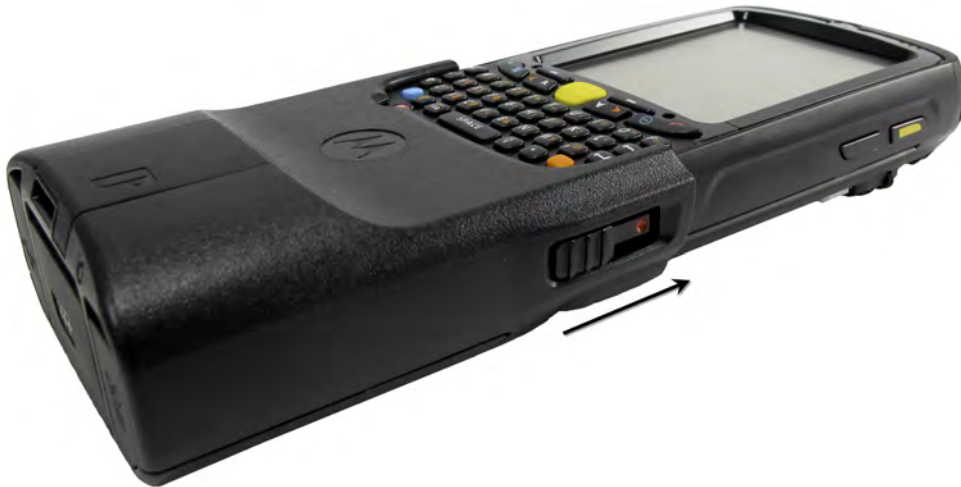
Figure 1-7 PDA and Security Adapter – Connected
