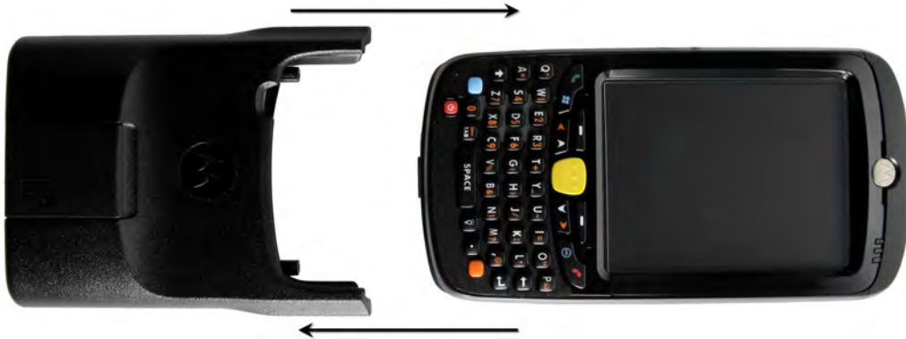
Figure 1-6 PDA and Security Adapter – Connecting
