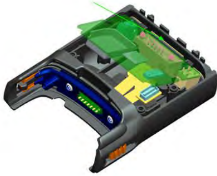
Figure 12-11 Assembling Front Housing – Connectors
