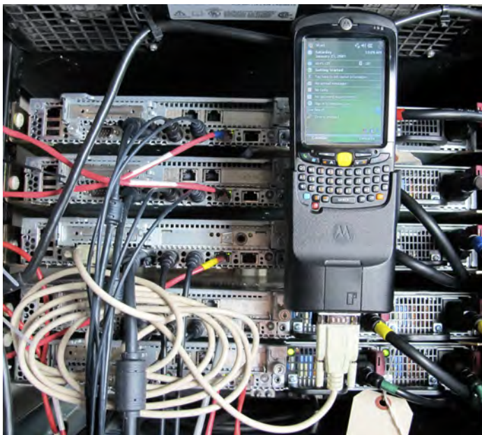
Figure 1-12 KVL and KMF – Direct Connection
