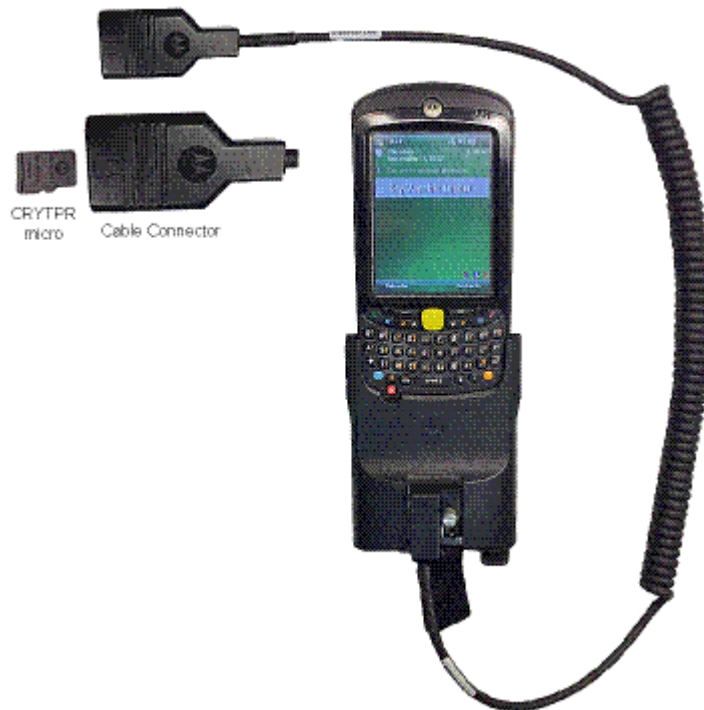
Figure 1-16 CRYPTR micro and KVL - Connected
