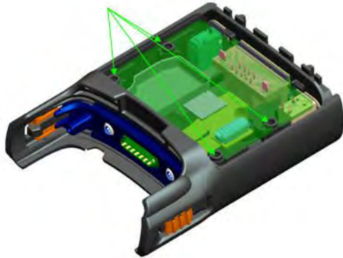
Figure 12-12 Assembling Front Housing – PCB Placed
