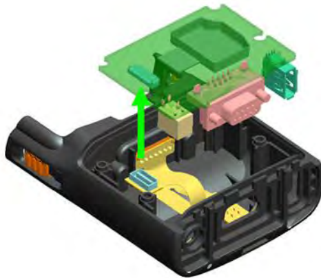
Figure 12-10 Assembling Front Housing – PCB
