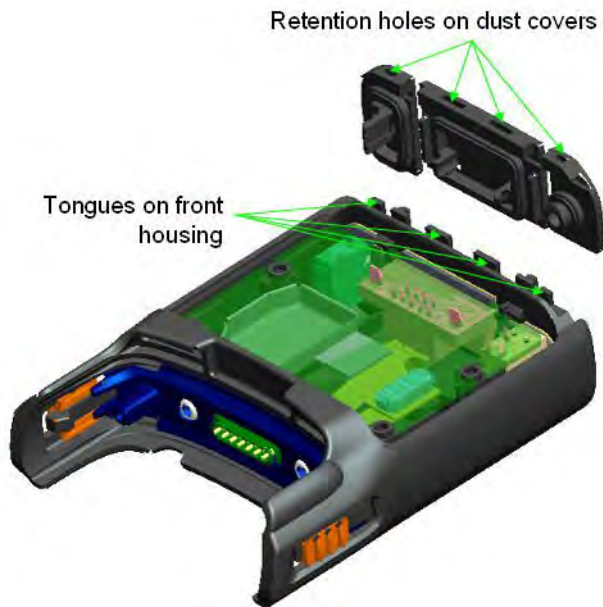
Figure 12-13 Assembling Dust Covers
