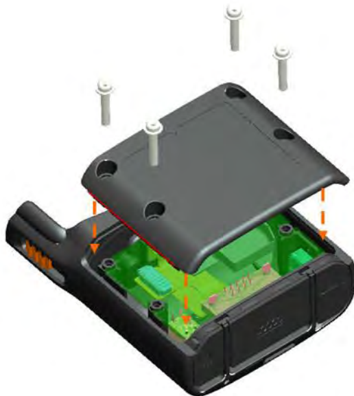
Figure 12-14 Assembling Back Housing to Front Housing
