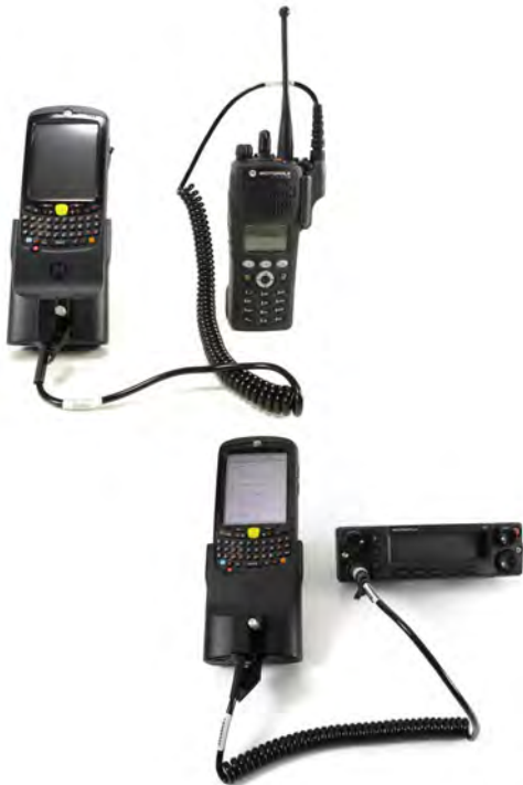
Figure 1-8 KVL and Radios – Connected (Example)
