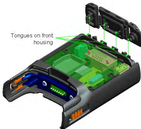
Figure 12-4 Removing Dust Covers
