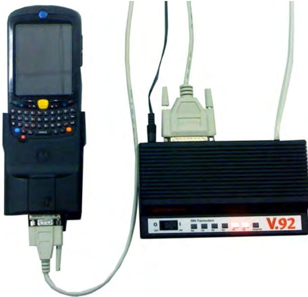
Figure 1-14 KVL and Serial Modem – Connected (Example)
