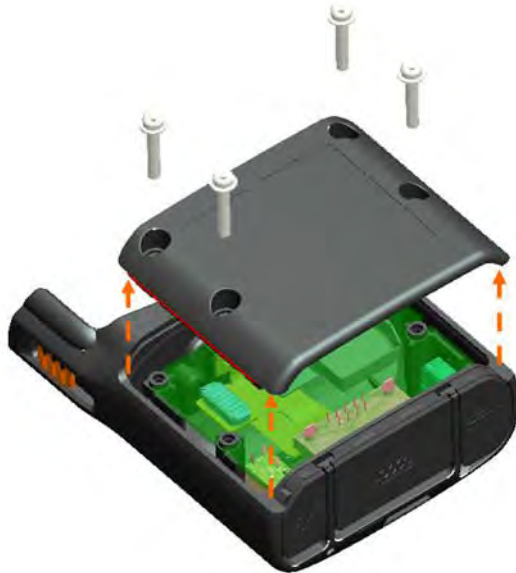
Figure 12-3 Removing Back Housing
