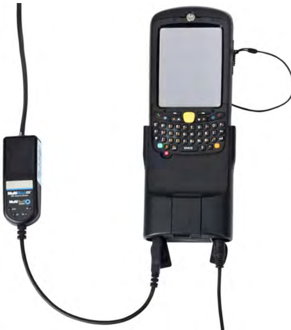
Figure 1-13 KVL and USB Modem – Connected
