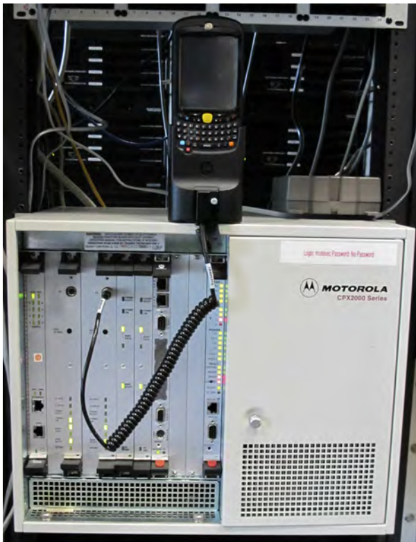
Figure 1-10 KVL and MEGEG – Connected (Example)
