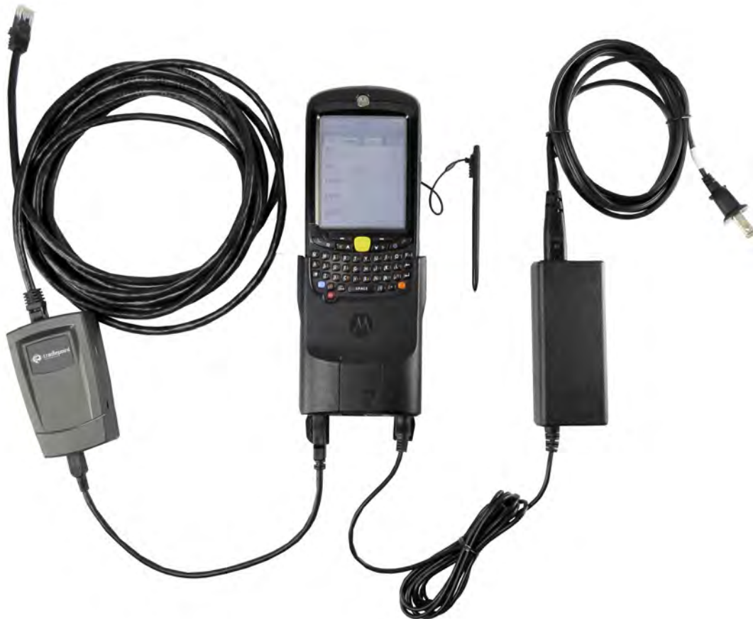
Figure 1-15 KVL and USB to Ethernet Adapter - Connected
