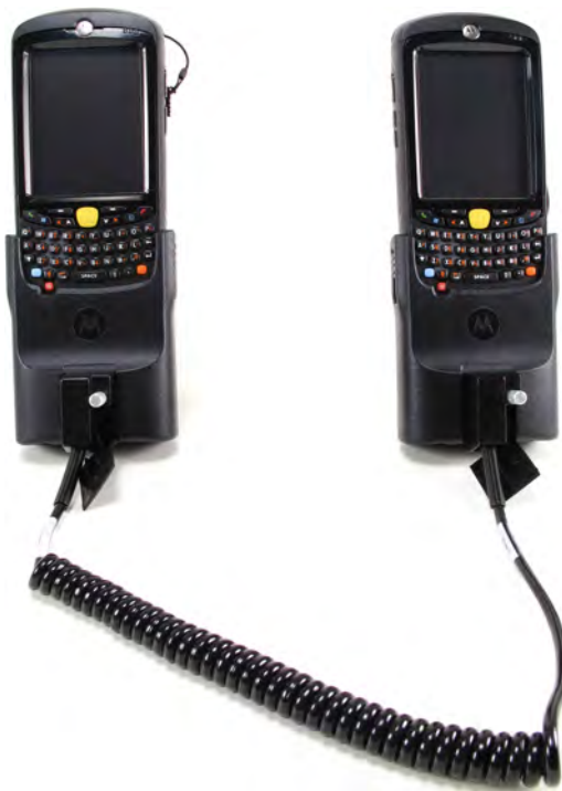
Figure 1-11 Two KVL Units – Connected
