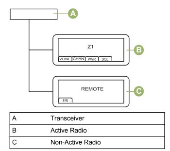
You can change the command between the 2 control heads by pressing the **Menu Select** button directly below F/R, or the **Menu Select** button preprogrammed user button on the keypad microphone.
