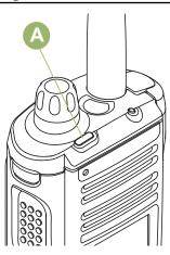
The Top Lightbar (A) indicates the secondary function of MFK and also the status of Intelligent Lighting.
