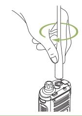
**3** To remove the antenna, turn the antenna counterclockwise.
