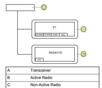
You can change the command between the 2 control heads by pressing the **Menu Select** button directly below F/R, or the **Menu Select** button preprogrammed user button on the keypad microphone.
