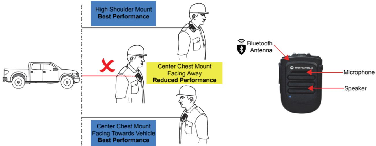
**For optimal performance, wear the WRSM high on the shoulder and facing the direction of the vehicle.**
