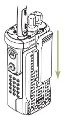
2 To remove the clip, use a flatbladed object to press the belt clip tab (<sup>(A)</sup>) away from the radio. Then, slide the clip upward and away from the radio.
