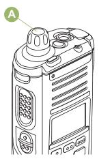
To increase the volume, rotate the On/Off/Volume Control Knob (<sup>®</sup>) clockwise.
