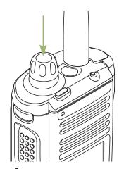
Rotate the **On/Off/Volume Control Knob** clockwise until you hear a click.
