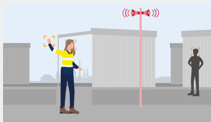
When a set gesture is detected, a voice alert sounds and immediate response is initiated.
