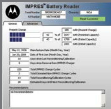
IMPRES BATTERY DATA READER, GENERAL INFORMATION SCREEN
