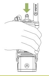
**3** To remove the radio from the carry holder, place the tip of your fingers on the ledge of the carry holder.
