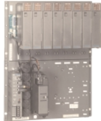
MOSCAD Rackmount RTU used as NFM RTU
