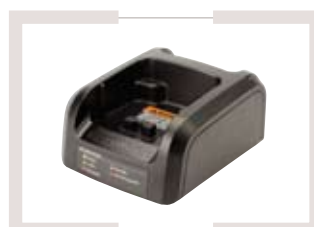
NNTN8234 Dual Desktop Charger base, supports simultaneous charging of radio and spare battery. Mini-USB port supports connection to Integrated Terminal Management (iTM) software and to download images and fingerprints from MTP6750 camera model. Power supply must be ordered separately.
