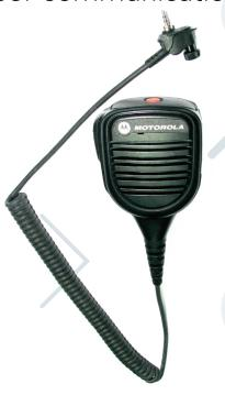
Remote Speaker Microphones (RSMs) are a vital two-way radio accessory solution for TETRA users who need to talk and listen without removing the radio from their belt or carry case. This RSM cancels out ambient noise to give MTP850 portable users the confidence of clear, understandable communication in noisy environments.
