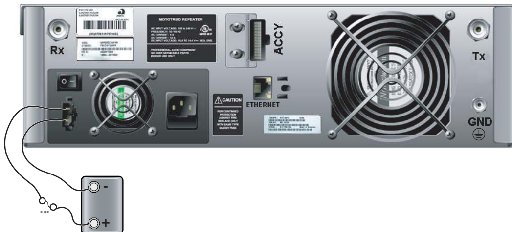
Figure 4-2 Making Connections to a Backup Battery
