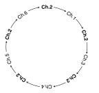
**Note:** Even though your radio has switched to a non-priority channel, your radio will still check for activity on the priority channel. If some activity is detected there, the radio will switch to that priority channel.
